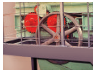
Close-up view of compensating gear train mechanism
