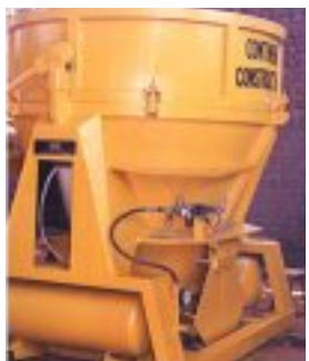
Pneumatically operated concrete buckets used in dam construction project.
