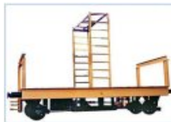
Dinky car for transportation of pneumatic concrete buckets for dam construction project.
