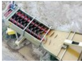
Screw lined with manganese steel liners for 150 TPH capacity Sand Washer / Classifier for Dam Construction Project.
