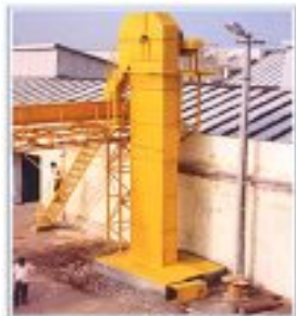
Belt type Bucket Elevator handling agro product at port site.
