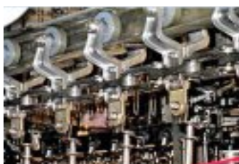
Close-up view of trolley of overhead conveyor
