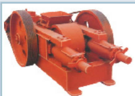
Small capacity plain roll crusher for crushing mineral material to - 2 mm size
