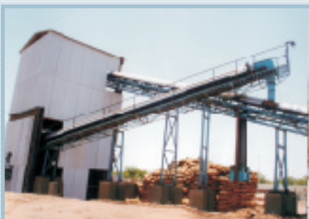
Recycling belt conveyor feeding oversize particles back to feed conveyor
