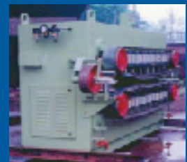
Caterpillar for haulage of high voltage power cable.
