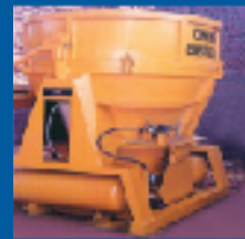
Pneumatically operated concrete buckets used at dam site.
