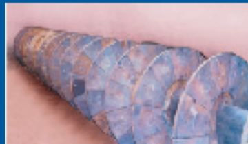
Manganese steel lined screw for sand washer.
