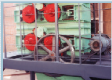
Four roll crusher with self compensating gear train mechanism
